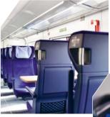
The seats have height-adjustable pillows and backrests that do not slide back when being adjusted, but instead slide into the seat frames, so that the seat behind is not adversely affected. Adjustable footrests and an individual reading light provide additional comfort in 1st class. The seat depth can also be adjusted. Each seat in 1st class and each double seat in 2nd class are equipped with power outlets.
